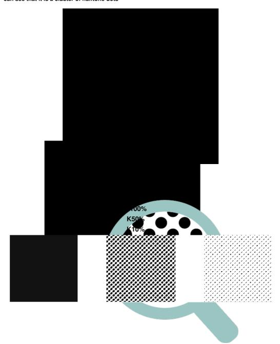
The saturation and size of the halftone dots will make an image appear darker or lighter
