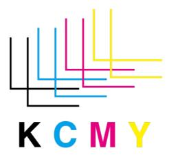
Trim Marks use registration colour to check for misalignment during printing. If any of the printing plates are misaligned, the colour ink will show which one, and we can make adjustments to re-align them.
